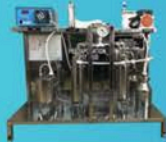
PERVAPORATION TEST SKID
