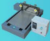
FLATSHEET MEMBRANE CASTING MACHINE
