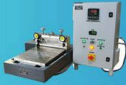
FLATSHEET MEMBRANE CASTING MACHINE WITH HEATING FACILITY
